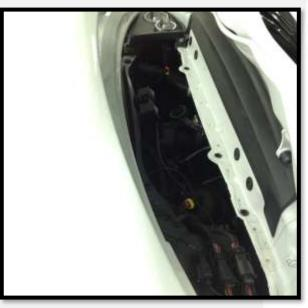
5. Remove spoiler base hardware. (x2) T30 bolts. Pushing forward on the very trailing edge releases the remaining clips. Spoiler base cover is now free. Lift up and tape to extended spoiler.
