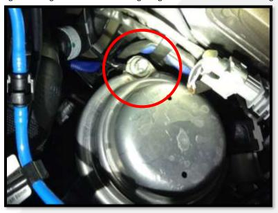
16. Suggested pluming and wire routing for a clean install. Secure with zip ties away from heat, rain water, and moving parts. Be sure to not rub on a sharp edge that can chafe through and cause future problems.
